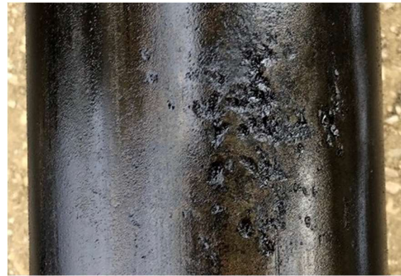
Figure 1 Stator Tube Corrosion – (a) normal surface corrosion; (b) structural corrosion.
