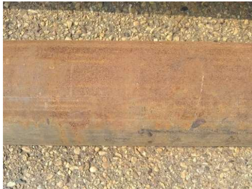
Figure 1 Stator Tube Corrosion – (a) normal surface corrosion; (b) structural corrosion.
