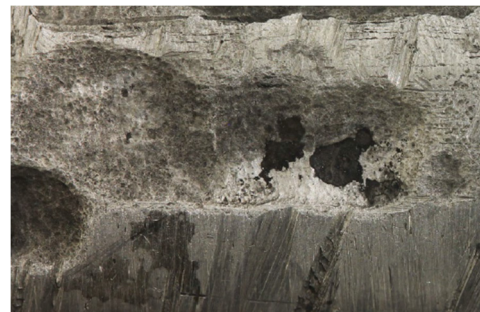
Figure 2, Characterization of the corrosion pits, deepest measured pit approximately 0.048"
