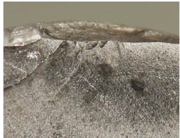
Figure 4, Closeup of the fatigue initiation point originating from the base of a corrosion pit
