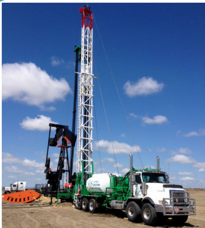
From initial well diagnostics to broken rod fish jobs and insert rod pump changes, the Lifting Solutions Rod Rig is extremely versatile and efficient in safely servicing conventional sucker rod wells.
