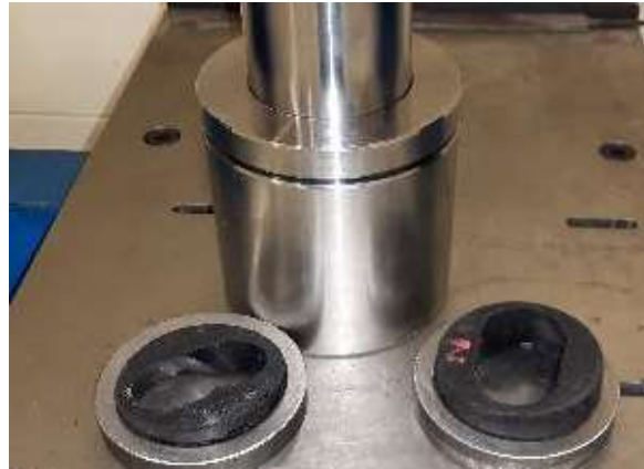
Figure 1: Bond Push-out Fixture & Pushed-out Bond Samples
