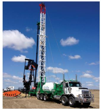
From initial well diagnostics to parted rod fishing jobs and insert pump changes, the Lifting Solutions Rod Rig is extremely versatile and efficient in safely servicing conventional sucker rod wells.
