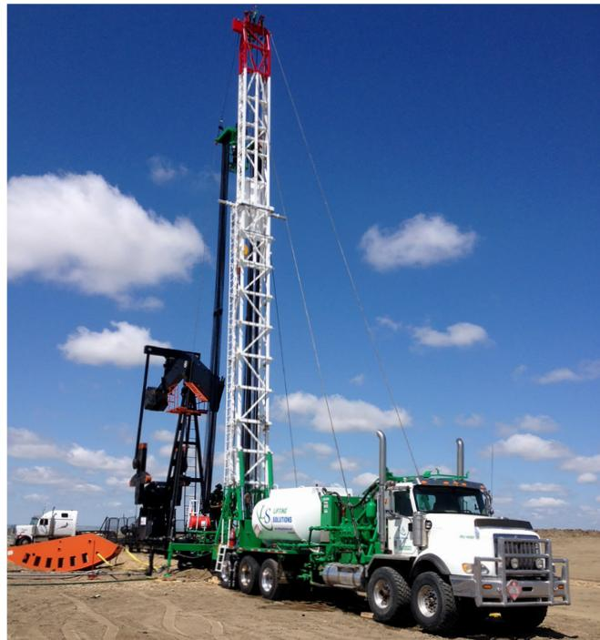
*From initial well diagnostics to broken rod fish jobs and insert rod pump changes, the Lifting Solutions Rod Rig is extremely versatile and efficient in safely servicing conventional sucker rod wells.*
