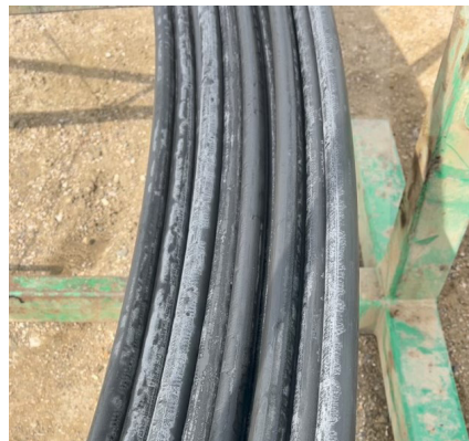
Surfaced KeBond after 174 days in operation (pulled due to tubing failure).
